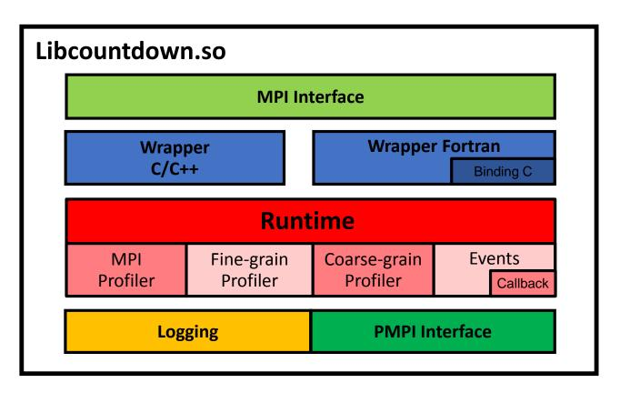
Figure 1: Logical view of COUNTDOWN components.
